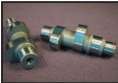
The Mackie cams were developed to complement the Mega-Sphere head. They provide a high 0.590-inch valve lift to take full advantage of port flow. Quick opening and moderate closing intake timing is part of the reason for the wide powerband.
