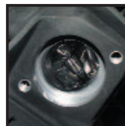
Mackie polishes the chamber and exhaust port (top) to reduce heat transfer while giving the intake port a brushed finish to enhance air/fuel mixing.
